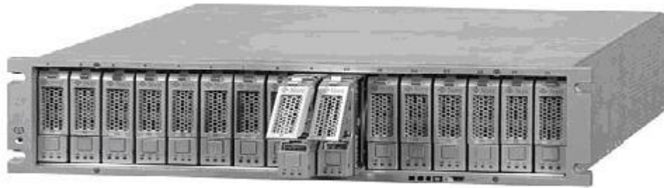
Figure 10.3 - A Typical Storage System of entry-level data (Sun StorageTek 6140)
